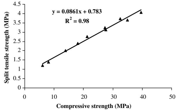
Fig. 4. Relation between compressive strength and split tensile strength of AS30 and BS30.
