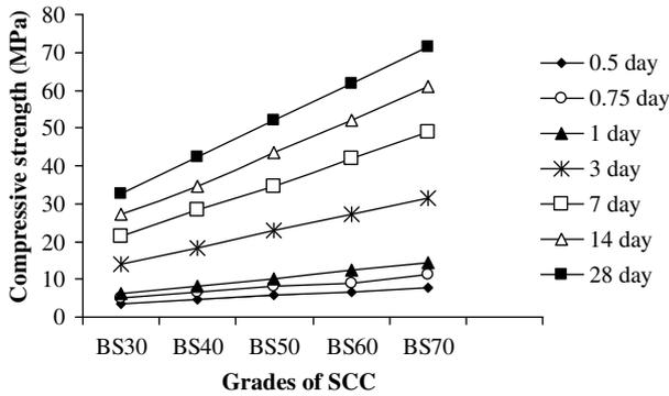
Fig. 2. Compressive strength of SCC (BS30–BS70) at early ages of curing.
