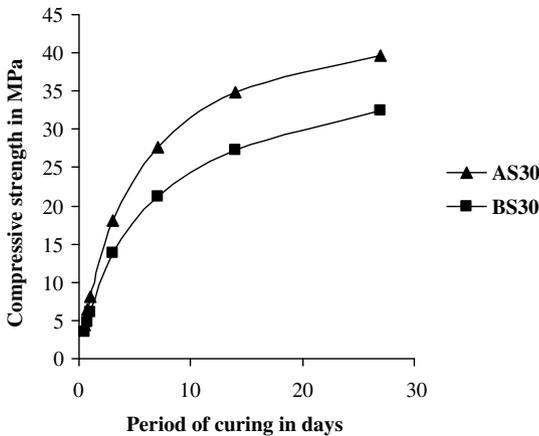
Fig. 3. Comparison of compressive strength of AS30 and BS30.
