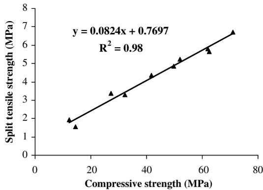
Fig. 7. Relation between compressive strength and split tensile strength of AS60 and BS60.
