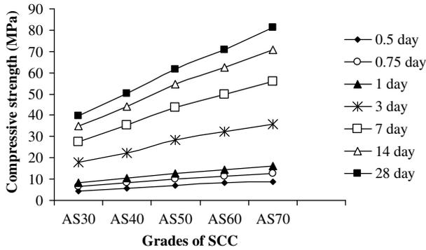
Fig. 1. Compressive strength of SCC (AS30–AS70) at early ages of curing.
