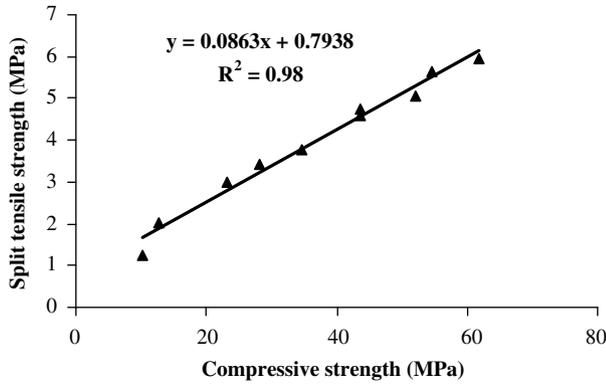
Fig. 6. Relation between compressive strength and split tensile strength of AS50 and BS50.
