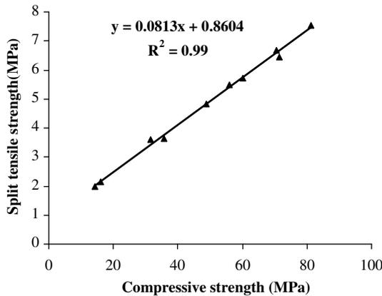
Fig. 8. Relation between compressive strength and split tensile strength of AS70 and BS70.
