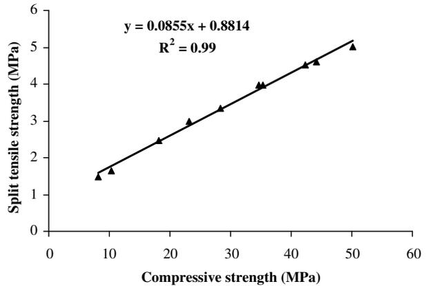
Fig. 5. Relation between compressive strength and split tensile strength of AS40 and BS40.
