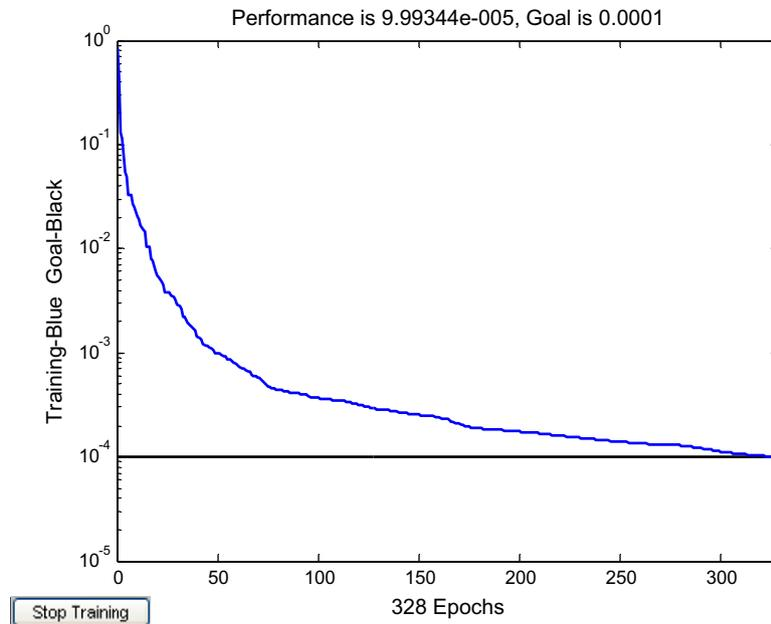
Fig. 13. Training performance for the Powell–Beale conjugate gradient backpropagation algorithm.
