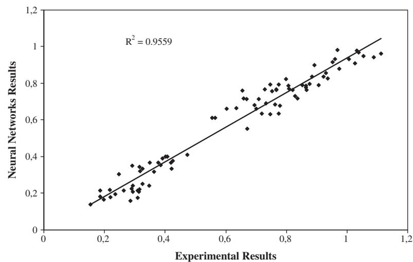
Fig. 10. Linear relationship between measured and predicted compressive strengths (the One step secant backpropagation algorithm).
