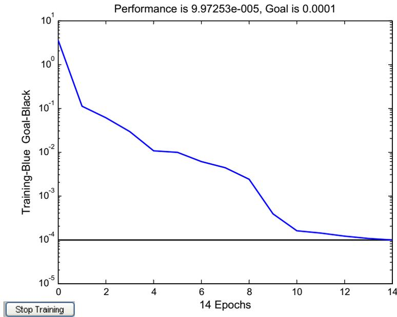
Fig. 11. Training performance for the Levenberg–Marquardt backpropagation algorithm.
