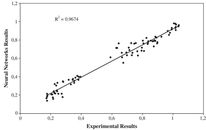
Fig. 8. Linear relationship between measured and predicted compressive strengths (the Fletcher–Powell conjugate gradient backpropagation algorithm).
