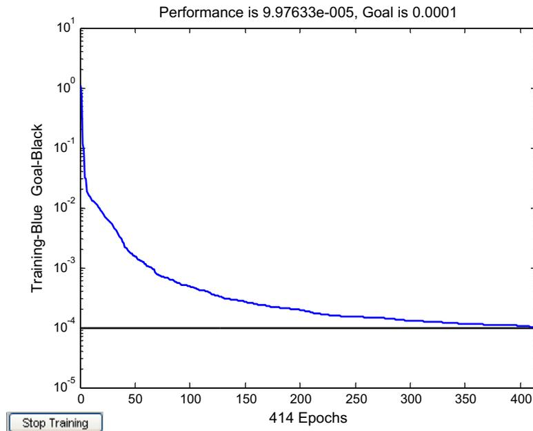
Fig. 15. Training performance for the Polak-Ribiere conjugate gradient backpropagation algorithm.
