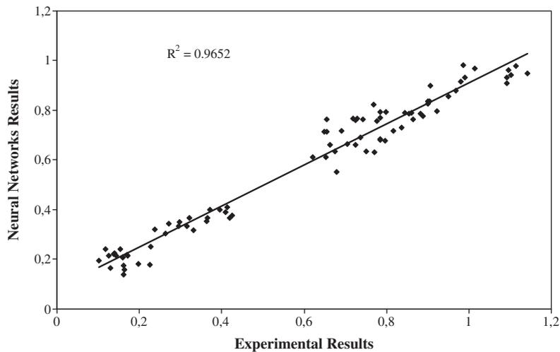
Fig. 7. Linear relationship between measured and predicted compressive strengths (the Powell–Beale conjugate gradient backpropagation algorithm).
