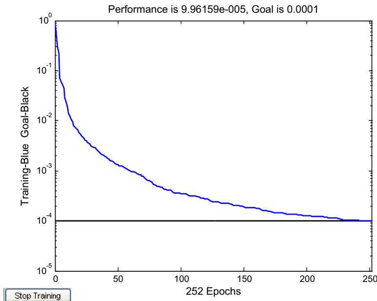
Fig. 12. Training performance for the BFGS quasi-Newton backpropagation algorithm.
