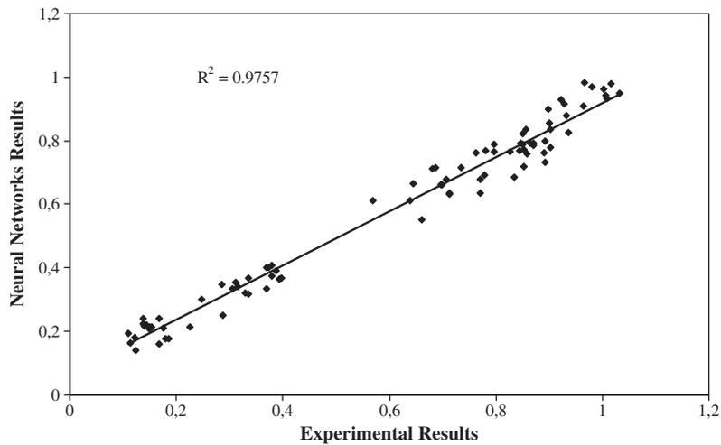
Fig. 6. Linear relationship between measured and predicted compressive strengths (the BFGS quasi-Newton backpropagation algorithm).
