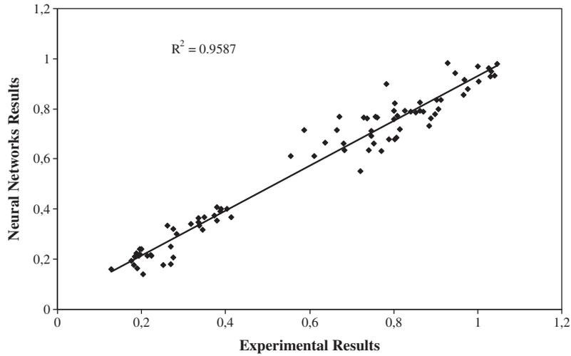
Fig. 5. Linear relationship between measured and predicted compressive strengths (the Levenberg–Marquardt backpropagation algorithm).
