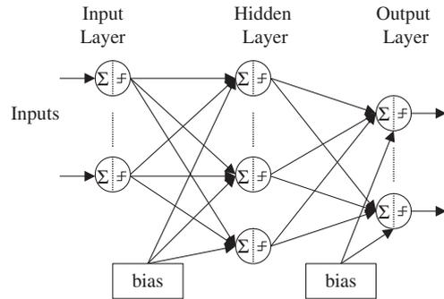
Fig. 3. Multilayer feed forward neural network structure.
