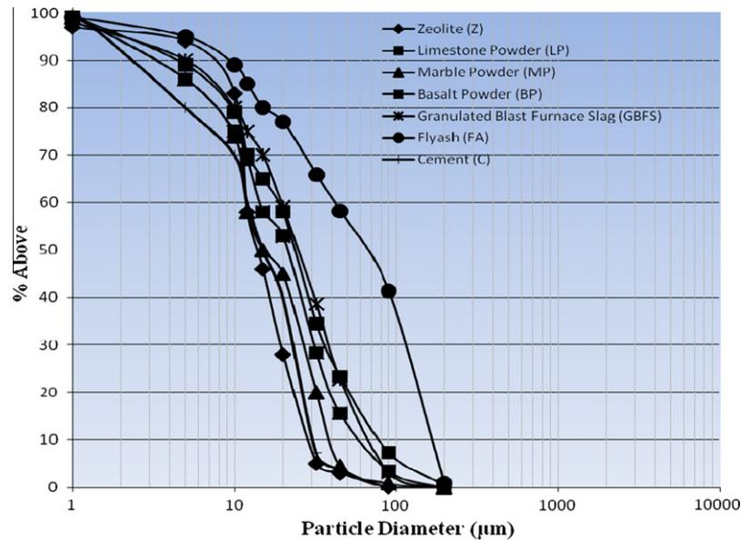
Fig. 1. The particle size distributions of mineral additives and Portland cement.
