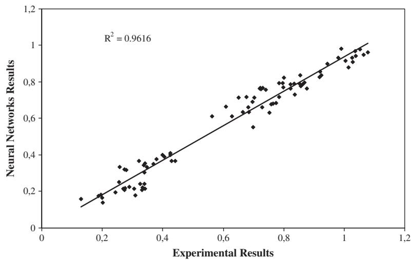
Fig. 9. Linear relationship between measured and predicted compressive strengths (the Polak–Ribiere conjugate gradient backpropagation algorithm).
