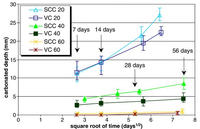
Fig. 5. Carbonated depth of concretes studied ( $t_0 = 28$  days).
