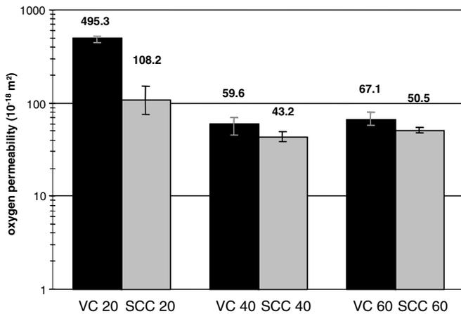
Fig. 3. Apparent oxygen permeability of concretes studied ( $P_{applied} = 0.2$  MPa, dry material).
