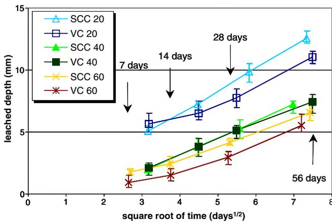
Fig. 6. Depth degraded by ammonium nitrate in concretes studied ( $t_0 = 28$  days).
