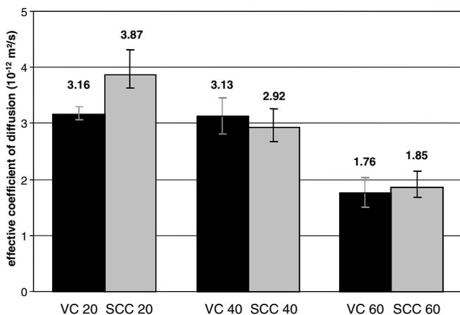
Fig. 2. Effective coefficient of chloride diffusion of concretes studied.
