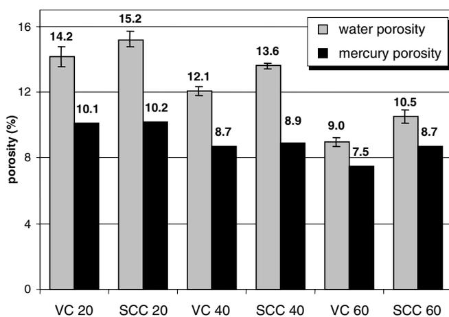
Fig. 1. Water and mercury porosity of concretes studied.
