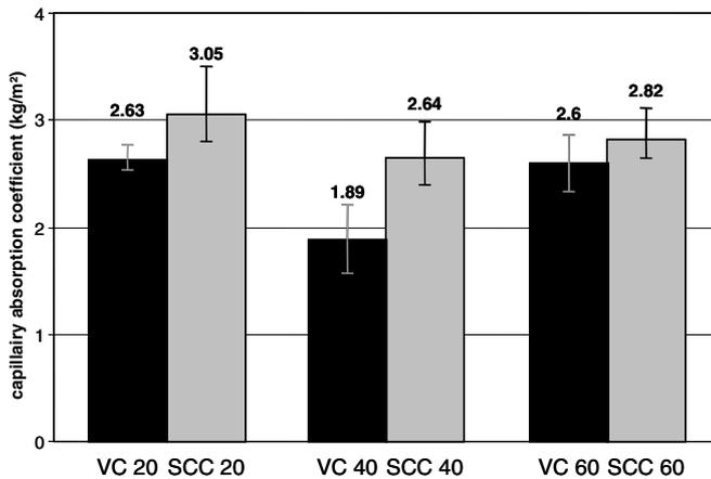
Fig. 4. Capillary absorption coefficient (at 24 h) of concretes studied.
