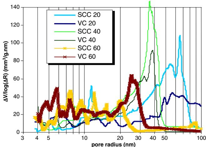
Fig. 7. Pore distributions of concretes studied.
