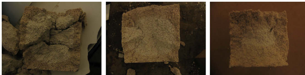
Fig. 13. Thickness of the absorbed water by G#3 after fire exposure: (a) 400-W-W: 6 mm (b) 600-W-W: 8 mm and (c) 800-W-W: 12 mm.
