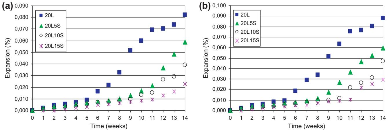
Fig. 9. Expansion values of mortars containing 20% limestone in (a)  $\text{Na}_2\text{SO}_4$  and (b)  $\text{MgSO}_4$  solution.
