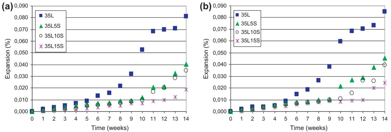
Fig. 10. Expansion values of mortars containing 35% limestone in (a)  $\text{Na}_2\text{SO}_4$  and (b)  $\text{MgSO}_4$  solution.
