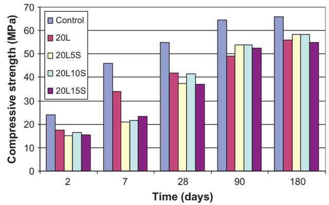
**Fig. 4.** Compressive strength values of limestone-silica fume mortars containing 20% limestone.
