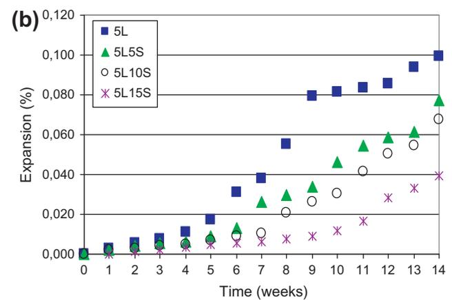
Fig. 8. Expansion values of mortars containing 5% limestone in (a)  $\text{Na}_2\text{SO}_4$  and (b)  $\text{MgSO}_4$  solution.
