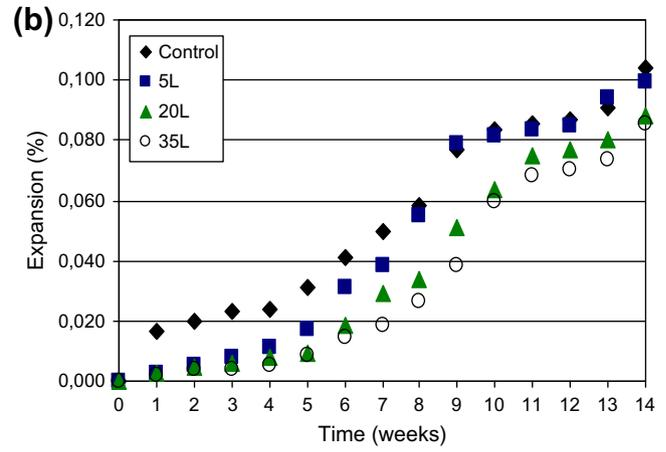
Fig. 6. Expansion of mortars containing only limestone in (a)  $\text{Na}_2\text{SO}_4$  and (b)  $\text{MgSO}_4$  solution.
