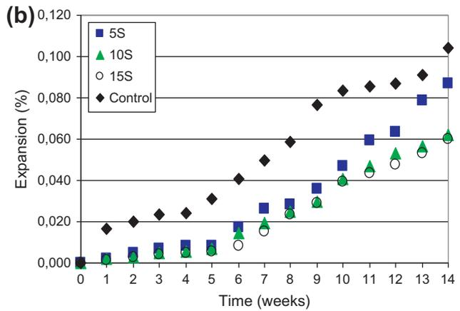
Fig. 7. Expansion of mortars containing only silica fume in (a)  $\text{Na}_2\text{SO}_4$  and (b)  $\text{MgSO}_4$  solution.
