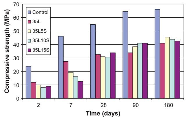
**Fig. 5.** Compressive strength values of limestone-silica fume mortars containing 35% limestone.
