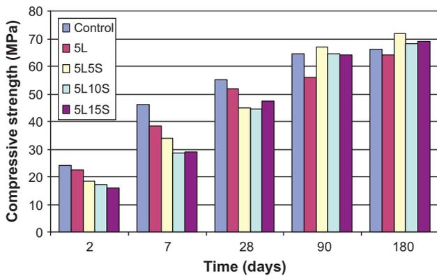
**Fig. 3.** Compressive strength values of limestone-silica fume mortars containing 5% limestone.
