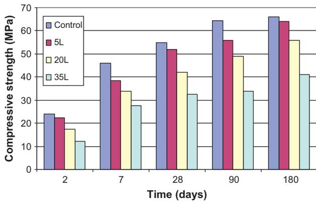
**Fig. 2.** Compressive strength values of mortars containing only limestone.
