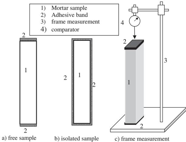
**Fig. 1.** Frame to measure shrinkage deformation.
