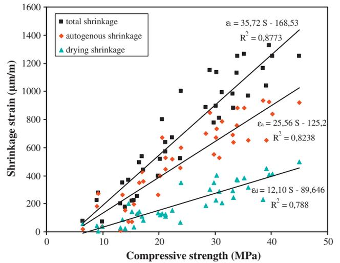
Fig. 9. Relationship between compressive strength and shrinkage. (ε<sub>t</sub>: total shrinkage, ε<sub>a</sub>: autogenous shrinkage, ε<sub>d</sub>: drying shrinkage, S: compressive strength, R<sup>2</sup>: coefficient of correlation).
