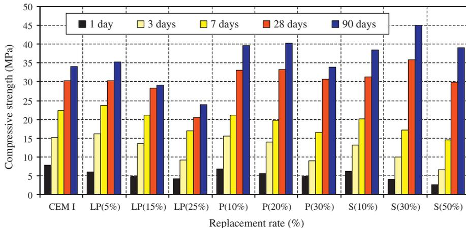
**Fig. 2.** Evolution compressive strength of mortars with various amounts of mineral additions (LP: limestone powder, P: natural pozzolan, S: slag).
