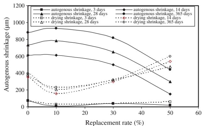
Fig. 8. Autogenous and drying shrinkage of mortars according to the replacement rate of slag.
