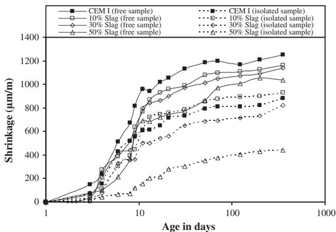
Fig. 5. Evolution of shrinkage for free and isolated samples of mortars with slag.
