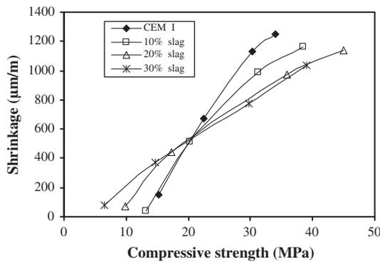
Fig. 12. Variation of shrinkage according to compressive strength for several replacement rate of slag.
