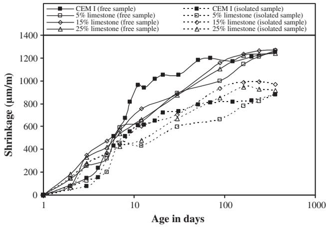
Fig. 3. Evolution of shrinkage for free and isolated samples of mortars with limestone powder.
