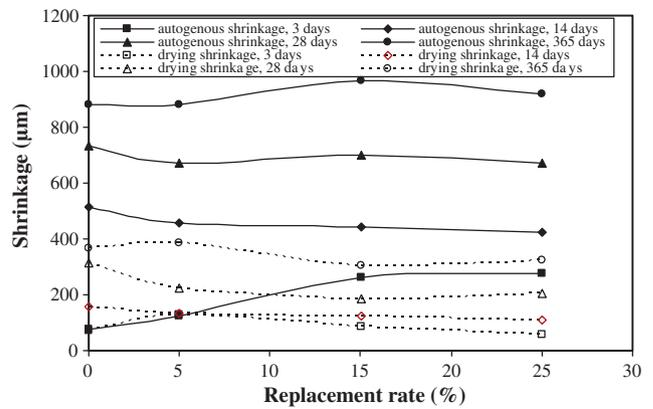
Fig. 6. Autogenous and drying shrinkage of mortars according to the replacement rate of limestone powder.
