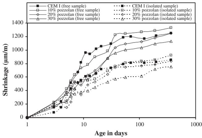
Fig. 4. Evolution of shrinkage for free and isolated samples of mortars with natural pozzolan.
