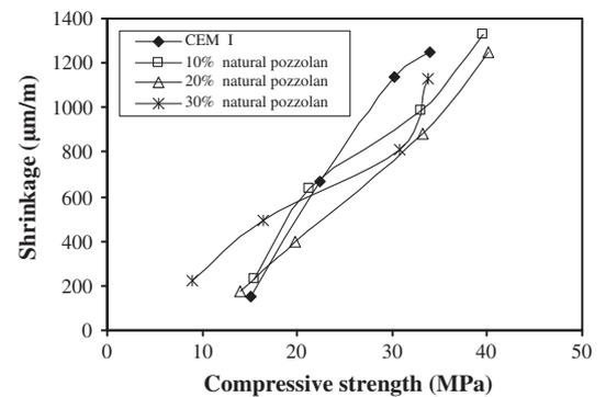
Fig. 11. Variation of shrinkage according to compressive strength for several replacement rate of natural pozzolan.
