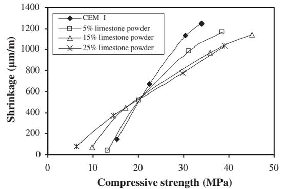
Fig. 10. Variation of shrinkage according to compressive strength for several replacement rate of limestone powder.
