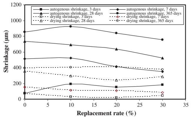
Fig. 7. Autogenous and drying shrinkage of mortars according to the replacement rate of natural pozzolan.
