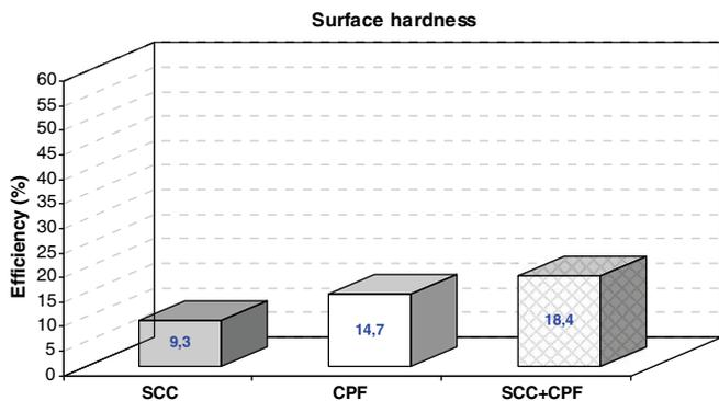
**Fig. 7.** Efficiency of SCC, CPF and SCC with CPF systems on surface hardness.
