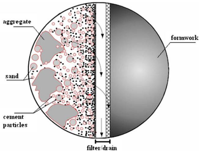
Fig. 1. Schematical representation of CPF functioning.
