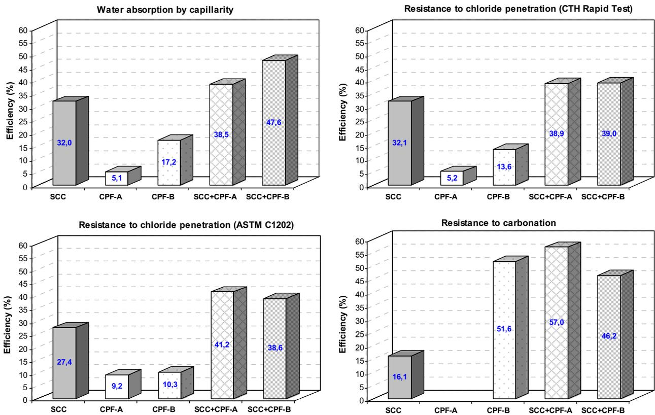
Fig. 9. Efficiency of SCC, CPF-A, CPF-B, SCC with CPF-A and SCC with CPF-B systems on durability properties.
