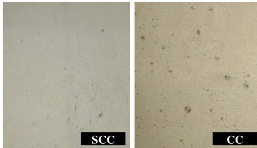
Fig. 4. Detail of concrete surfaces resulting from SCC and CC.
