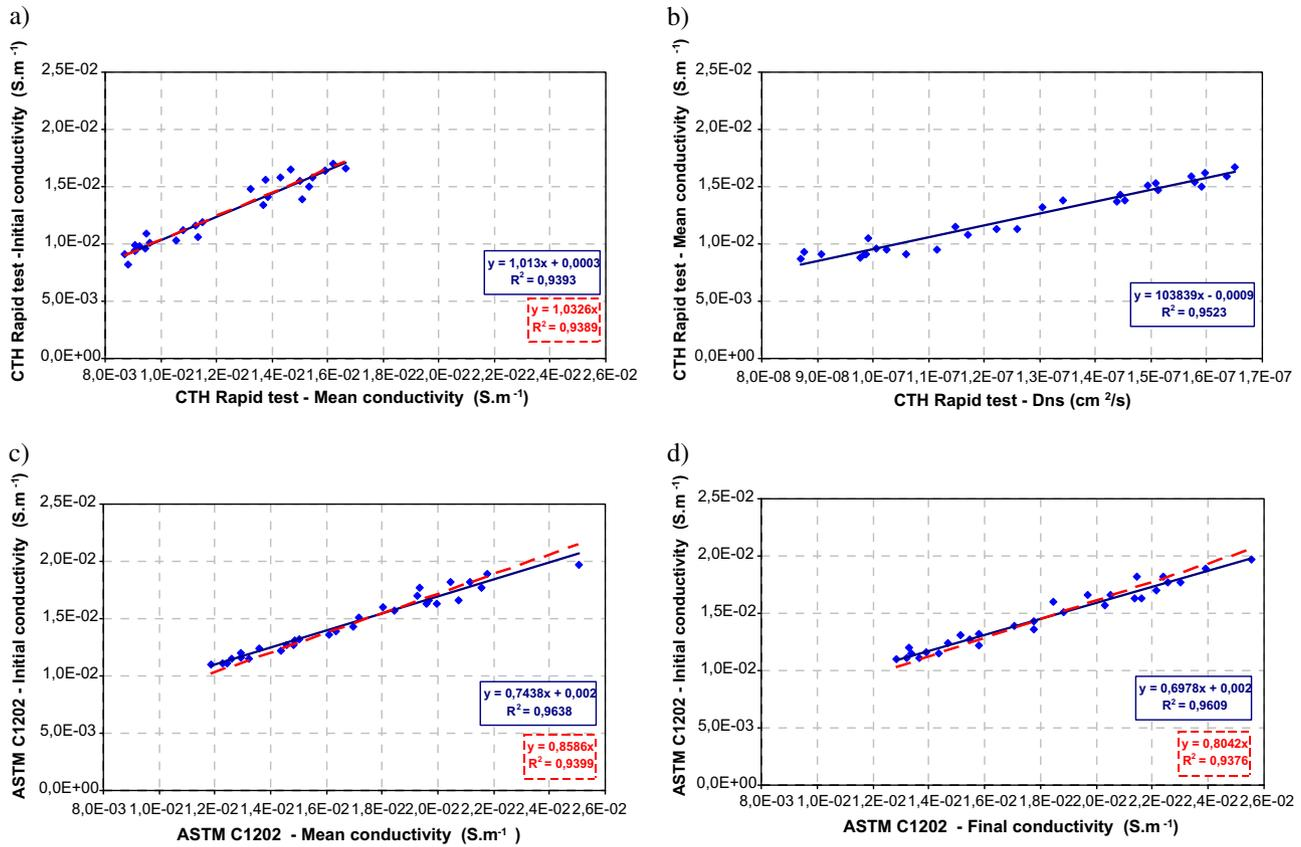
Fig. 8. Correlation between results of CTH Rapid test and ASTM C1202 test.
