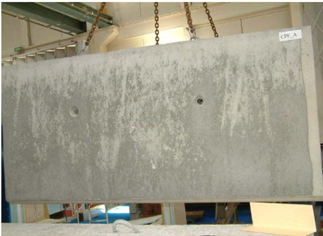
Fig. 5. Concrete surfaces resulting from application of CPF-A on CC box-culvert.
