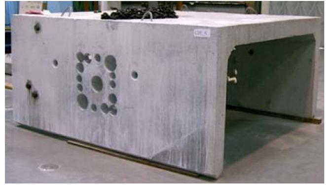
Fig. 3. Box-culvert and location of test cores in side wall A.
